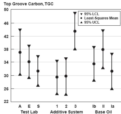
The CI-4 tests go on to demonstrate further these interactions between additives and base oils.
