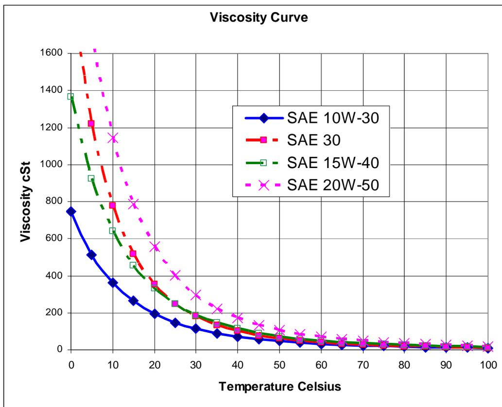
You can see from this chart that until the engine reaches operating temperature there is very poor lubrication and frequently the oil is going through the bypass valve directly to the bearings without passing the filter (in other cars it goes through the dirty filter and out the bypass valve). During this period you should refrain from putting the engine under high load or high rpm.
