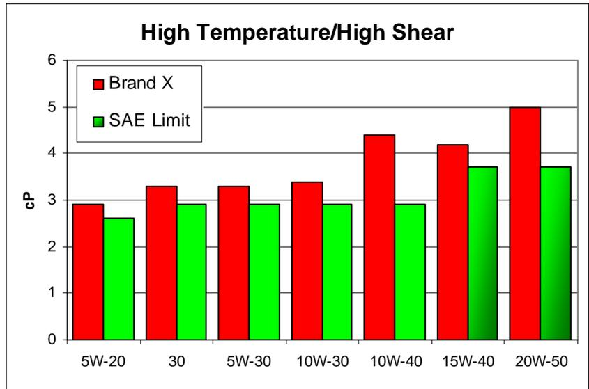
In this example, the Brand X 10W-40 is synthetic. It therefore behaves like a SAE 40 under stress.
