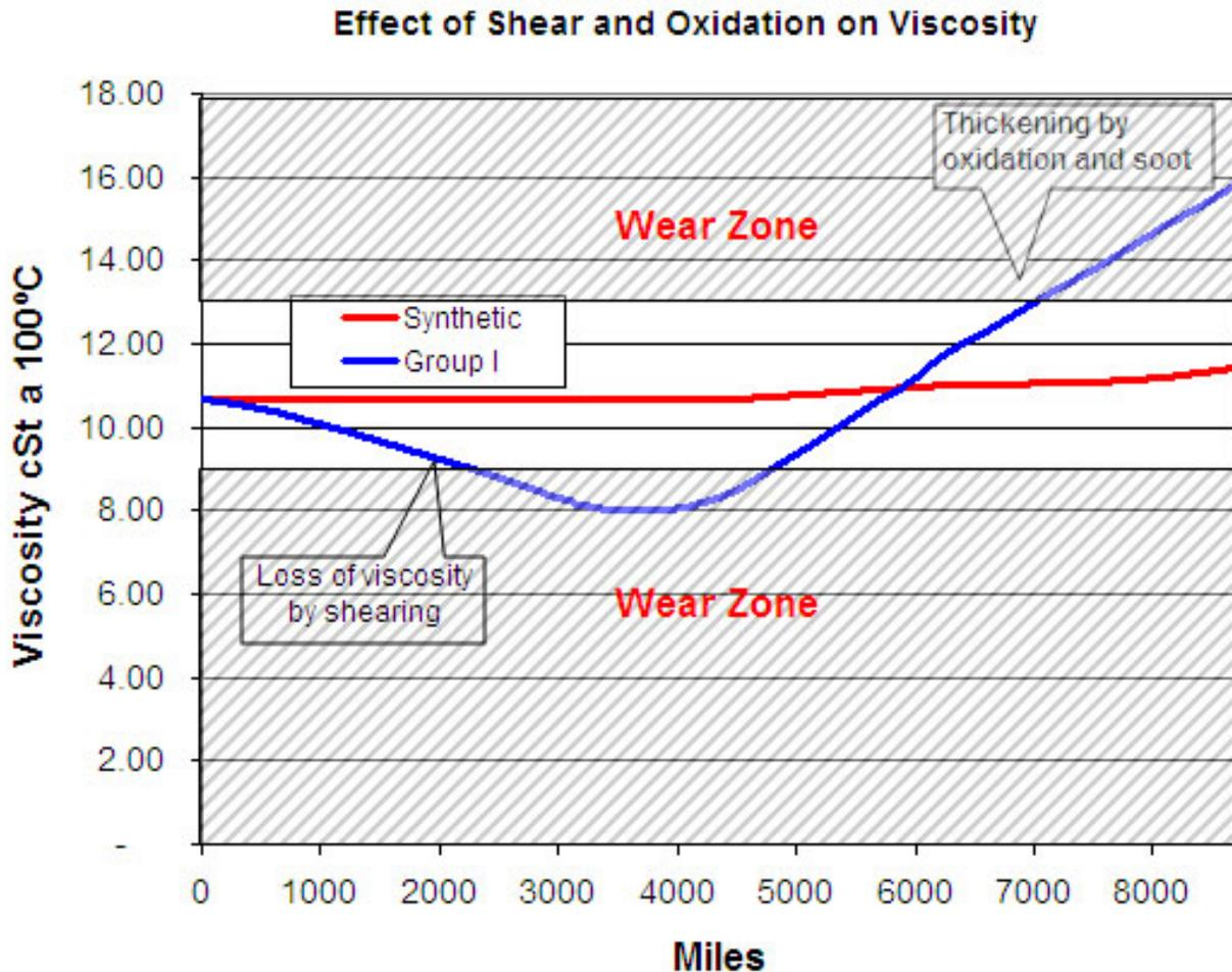
In engines that depend on gears for timing (rather than timing belts and chains) there is often a tendency to shear at a very high rate. This is not as big a problem in Corvairs because the timing gears are larger in diameter, slowing their contact and milling action.
